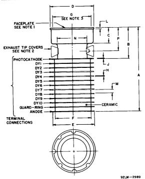
The dimensions in millimeters are derived from the basic inch dimensions (1 inch = 25.4 mm)
